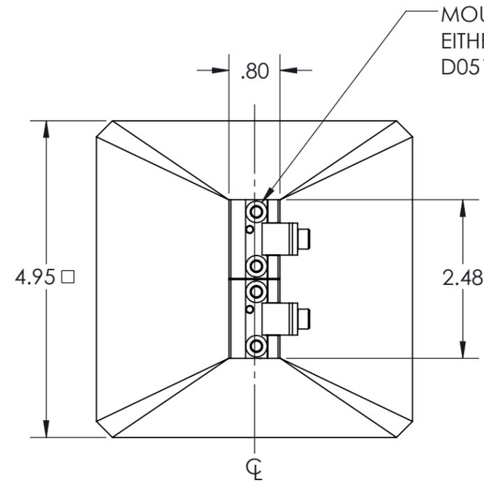
MOUNTING HOLES CAN ACCOMMODATE EITHER ONE D05125 CENTERED OR TWO D05125 FIXTURES MOUNTED IN PARALLEL AS SHOWN
